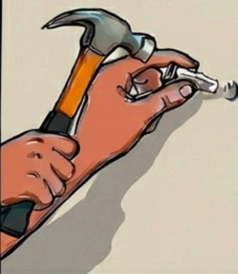
For holes with no studs behind them, gently tap the provided plasterboard anchors into place using a hammer.
