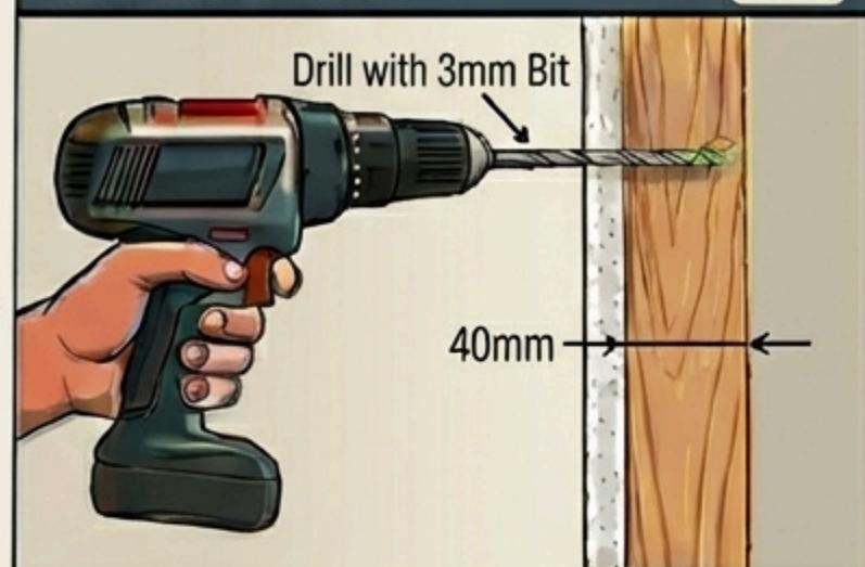
Remove panel. Drill holes at marked positions. For studs, ensure 40mm depth.
